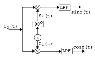
Figure 6: Oscillator offsets with reference signal.
