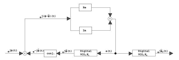
Figure 7: Modified baseband Costas loop for frequency-locking.
