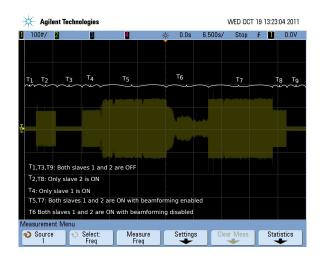
Figure 10: Received signal amplitude at the receiver - I.
