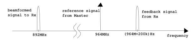
Figure 5: Frequency multiplexing scheme for beamforming experiment.
