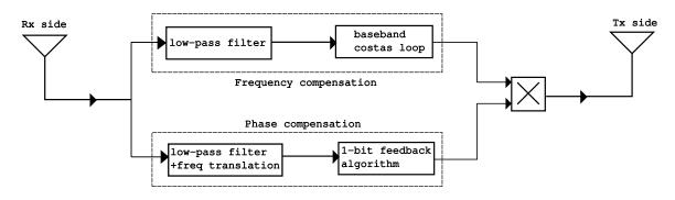
Figure 4: Signal processing at the Slave nodes.
