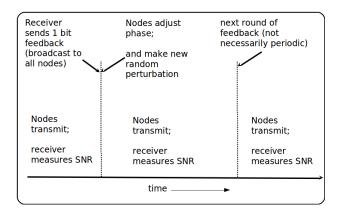
Figure 3: Illustration of the 1-bit feedback algorithm.
