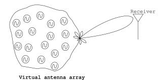
Figure 1: Energy efficient transmission using distributed beamforming.
